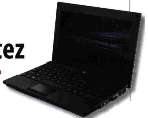
Intel Core 2 Duo T6570 (2,1 GHz), FSB 800 MHz, 2 MB Caché L2, 2 GB de RAM (DDR3 a 1.066 MHz), HD 2,5" 250 GB SATA 7.200 rpm, GPU Intel GMA 4500MHD.
